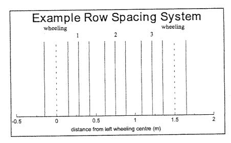
The form produced when selecting the Spacings sub-menu item is shown on the next page. This form requests the user to supply details related to the spatial pattern of plants. To illustrate its use, reference is made to an example row spacing system, illustrated here. There are three groups containing three each The distance rows. between groups (outer row to outer row) is 0.2
